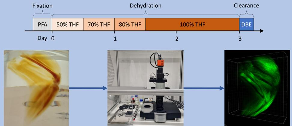
**Figure 2. fDISCO and light-sheet imaging.** PFA: paraformaldehyde, THF: tetrahydrofuran, DBE: dibenzyl ether, fDISCO: 3D imaging of solvent-cleared organs with superior fluorescence-preserving capability. Imaged at OJ2 microscope core facility, VU University Medical Center Amsterdam.
