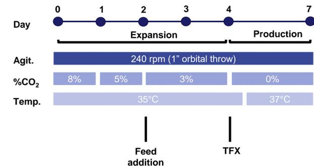
Figure 1: Ultra scale-down AAV manufacturing process overview.
